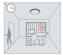
If there is no more movement, the light turns off automatically after hold-time preset.
