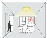
With movement and insufficient ambient lux level, the light is triggered on 100% by the detector.
