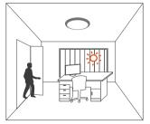
The light keeps off during daytime even when movement is detected. (Ambient lux level is above preset daylight threshold)
