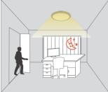
With movement and insufficient ambient lux level, the light is triggered on by the detector.
