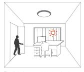
The light keeps off during daytime even when movement is detected. (Ambient lux level is above preset daylight threshold)
