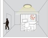
If there is no more movement, the light dims to stand-by dimming level after hold-time.
