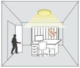
With movement and insufficient ambient lux level, the light is triggered on by dimming the detector.
