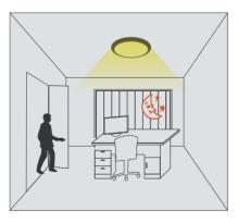
With movement and insufficient ambient lux level, the light is triggered on by the detector.
